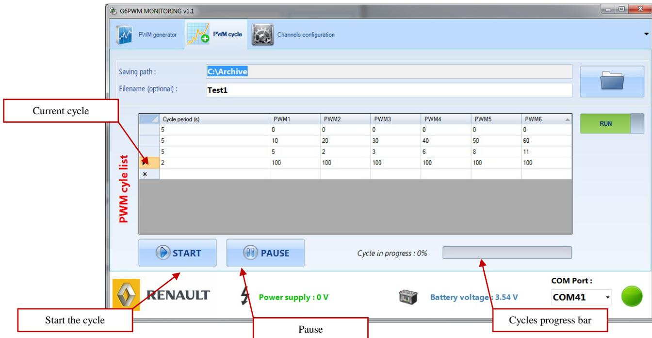
Creating a program is very straightforward. First the time of how long each PWM generation can last (in seconds) has to be set then the PWM values of each channel can be filled.
