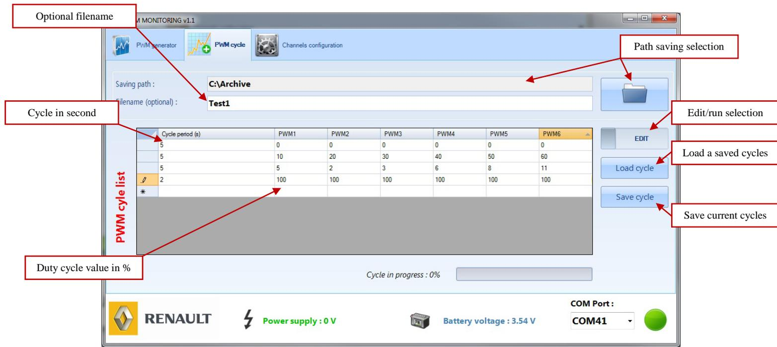
**SAVING PATH:** user must configure a “Saving Path” before starting a cycle and record measurements.
