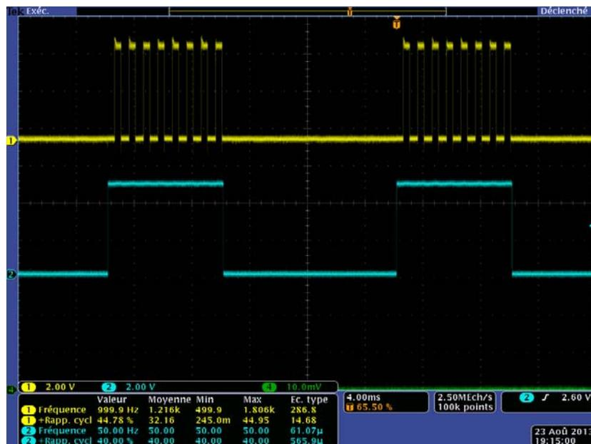
The signal generated by the G6PWM in this example is 50Hz 40% PWM ratio TTL (in blue) and the read back when the level is high is 1KHz 45% PWM ration (in yellow).
